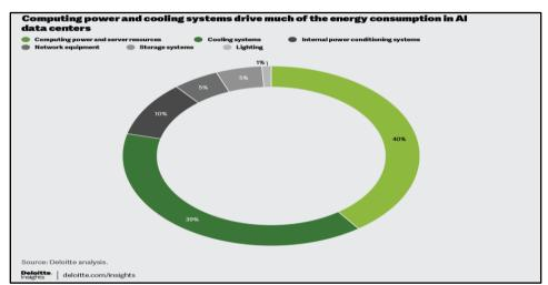
Computing Power & Cooling Energy Consumption in AI Data Centers
